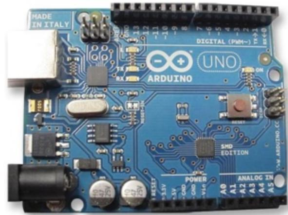
Figure 3. Arduino Uno microcontroller
